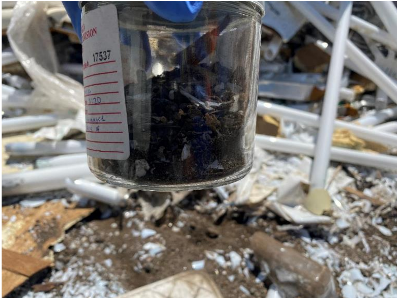
Sample is soil, debris and broken glass from bulbs
